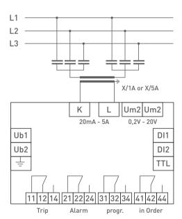
Max. output rating DC (ohmic) 30 V / 5 A; 60 V / 1 A; 110 V / 0.5 A; 220 V / 0.3 A
