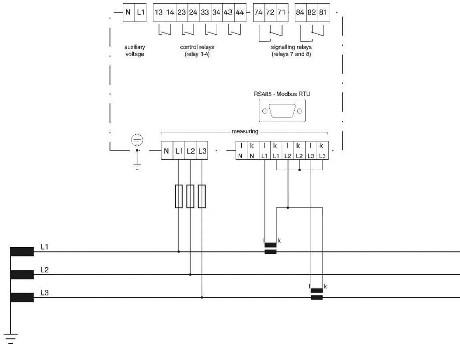
**5.5 3-phase measurement with three current transformers and measured neutral conductor current (four-wire measurement)**
