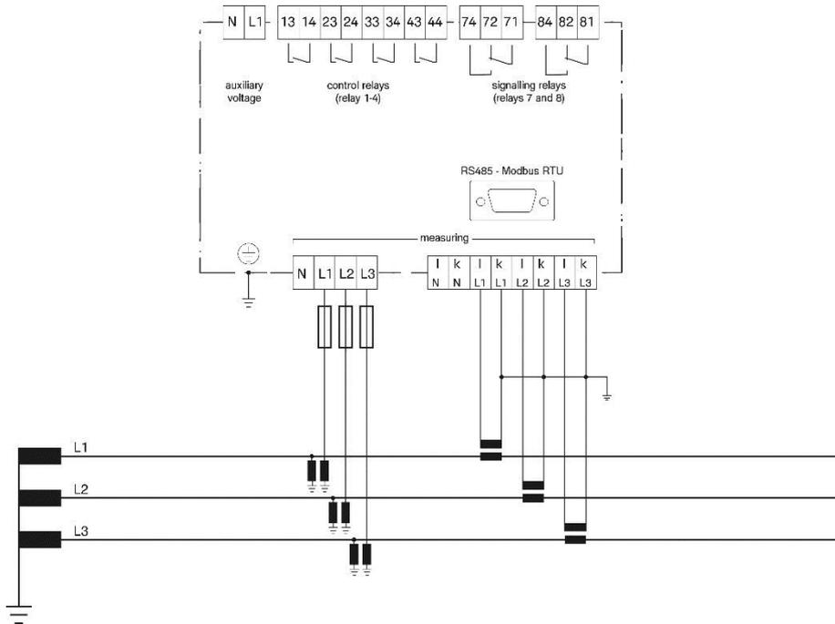
**5.3 3-phase measurement with two current- and three voltage transformers (three-wire measurement)**
