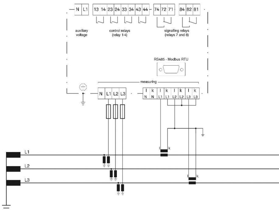
**5.4 3-phase measurement with two current transformers (three-wire measurement)**
