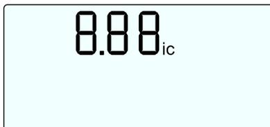
The first line of the main window shows the current  $\cos \varphi$ . A small **i** or **c** indicates whether the  $\cos \varphi$  is **inductive** or **capacitive**. In the respective submenus, this line shows the name of the current item.
