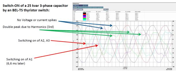
The BEL-TS Beluk thyristor controller is characterized by fast and low-reaction switching behavior.
