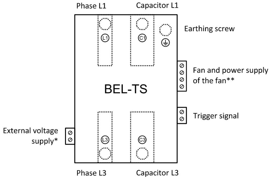
\* Depends on the thyristor type. This connector is only available on devices with an external power supply.
