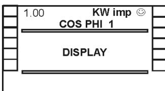
**Cos φ, valid Target cos φ (1 or 2):** Showing of power-factor and of the active target power factor (e.g. tariff switching with digital input).
