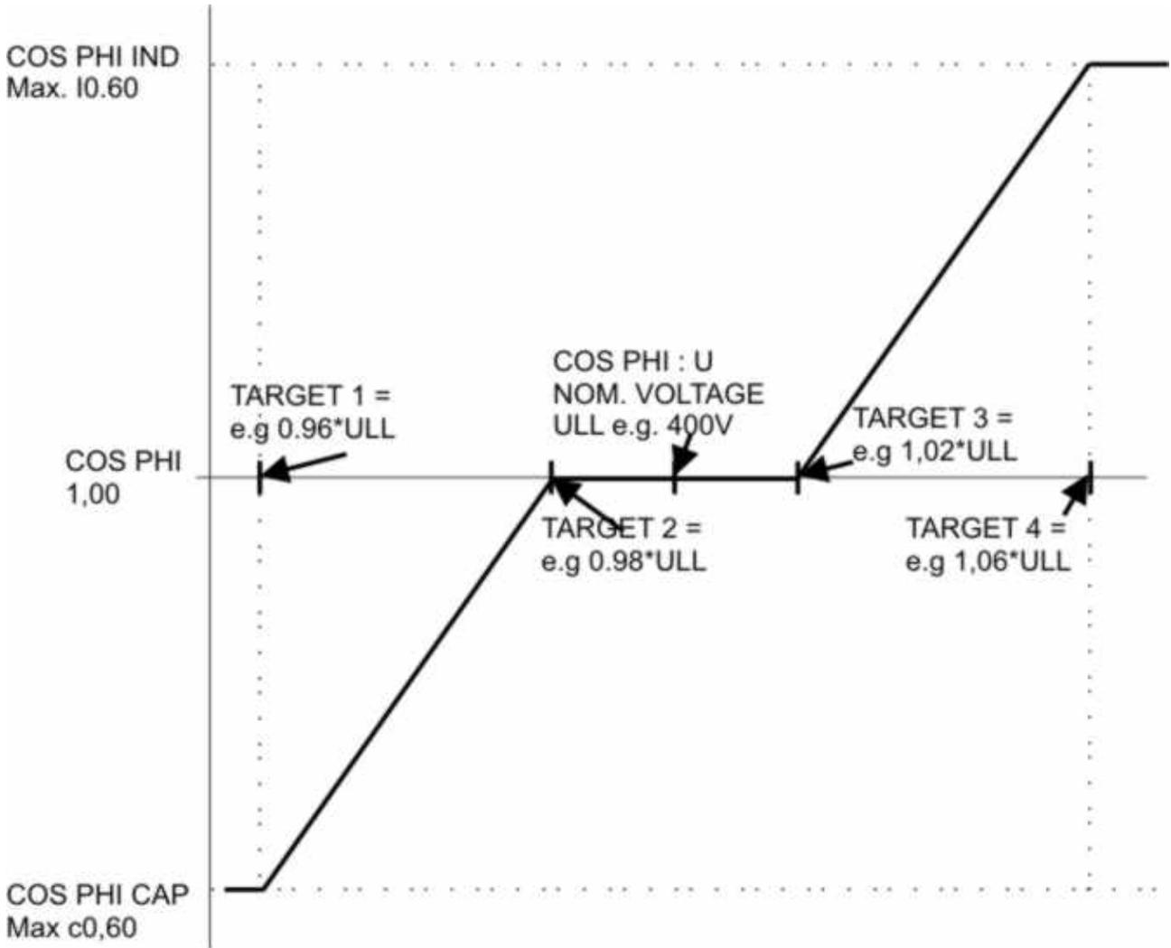
**Regulation mode normal algorithm:** 4 different regulation modes are available at BLR-Q(U) for standard cos phi control, in voltage control this settings does not work:
