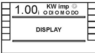
**Cos φ, DI, M, DO:** Display of power factor and status of inputs and outputs (○=inactive, ●=active)
